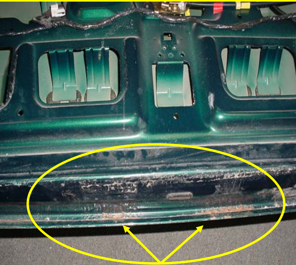
Rust Throughout Replacement Part
