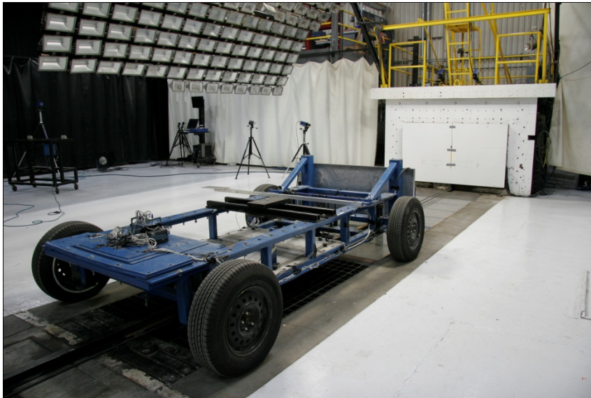
FMVSS 214 simulation vehicle and barrier.
