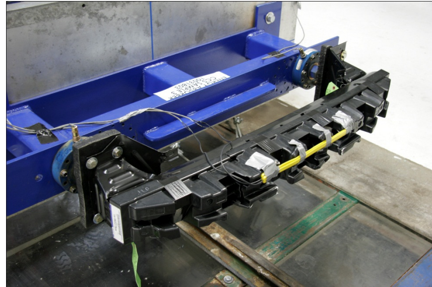
Ford Fusion reinforcement bar and energy absorber
