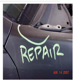
All parts that are to be repaired will be circled & the word "repair" printed next to it.
