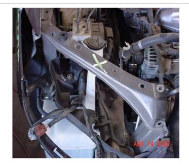
$\label{eq:all-parts} \mbox{ All parts that are to be replaced will} \\ \mbox{ be marked with an } X$
