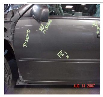
All parts that are to be Removed & Reinstalled will be marked with the letters R&I with an arrow pointed to them.
